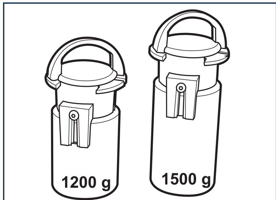
Figure 21: Typical Weigh Scale Fixtures
